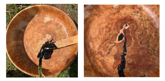
Blackwood is a fast-curing paste used for filling cracks, cavities, and other irregularities in wood.
