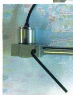
Insert camera housing onto long 12mm bar and tighten down the grub screw to fix in place.
