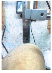
I have found that if you place the camera about 3-4 inches away from your hollow form, the image is a nice size to work with. Too far away, the image is too small. Also aim for the cutter in the middle of the screen.
