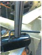
Use allan key to screw 16mm main stem onto hollowing jig. Its best to use a little thread lock or 2 part epoxy resin, and leave it on as a handle even if not using the camera!
