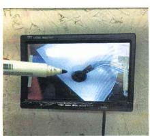
Draw with the white board marker provided, the image of the cutter. I use a circular motion. You need to be as accurate as you can. If you make a mistake, just rub it out. There is 2 screen protectors on the screen. Take care not to press too hard on the screen when rubbing out. Use a thinners or white spirit to wipe off.
