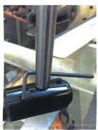
Use allan key to screw 16mm main stem onto hollowing jig. Its best to use a little thread lock or 2 part epoxy resin, and leave it on as a handle even if not using the laser!
