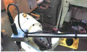
With laser pointing down, add the power extension lead onto the horizontal bar. Use the cable ties provided to secure. Ensure you loop enough on the laser. The second is placed about 6" away from the head
