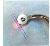
Adjust laser point by twisting the head of the laser. This will focus the point. Then adjust the arm so that the setting is at required distance to cutter (this will be the wall thickness) So for 5mm wall thickness use guide lines to set.
