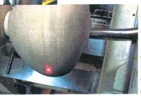
As you cut, the dot will move towards the outside shape. Remember where the dot is in relation to the cutter. You will need to adjust for the top of the hollow form and then to go down the side (depending on shape)
