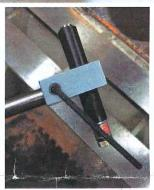
Insert laser housing onto long 12mm bar and tighten down the grub screw to fix in place.
