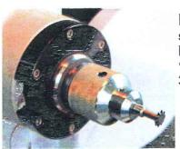
HOPE lathe spindle holder. M33x3.5, 1"x8, 1 1/2 x 6 and 3/4 x 16 available.
