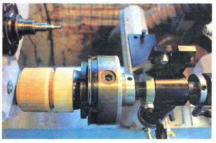
Now lift back again using the hinge plate to check your thread. If you have made the spigot 100% the correct size the threads should work. But don't worry if the threads are still tight. If they are follow the next steps on page 8
