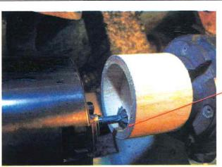
MAKE SURE: the chuck is tight on the threading jig. The jig is 90 deg to the banjo (makes it easier to line up parallel) Ensure the stem of the threading jig is fully locked down.
