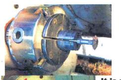
Using pin jaws on another chuck works fine.
