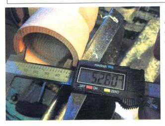
Use a set of vernier to measure the tips of the female threads. Wobble the verniers slightly when touching the threads to ensure you have maximum diameter but not so much pressure that you damage the threads. On the sample it is 52.8mm
