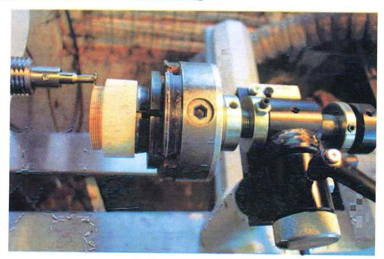
Next swing the jig back into the cutting position making sure the jig is wound back so it clears the cutter. Add an extra click, then re-cut. Repeat until you have taken enough down to make your perfect thread.
