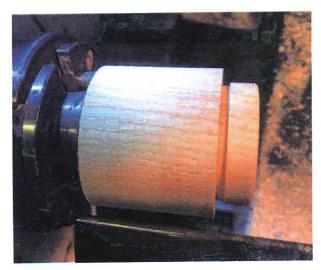
Turn the male spigot to exactly the correct size. This will ensure that the thread will fit first time. Make a shoulder relief cut about 3mm wide and deep so the thread cuts into this space.
