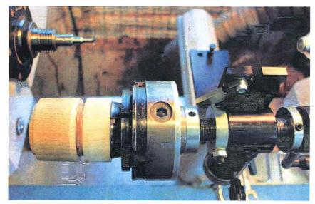
Now you can use the hinge plate to check. Ensure the cutter is clear, undo the front lever and lift the jig and chuck towards you. This will allow you to check the fit. It should still be tight but sometimes the box may fit at this stage. Its good to check.
